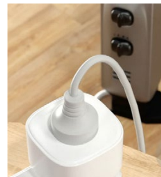
Figure 2.2: Meross smart energy monitor for daily energy consumption logging.
